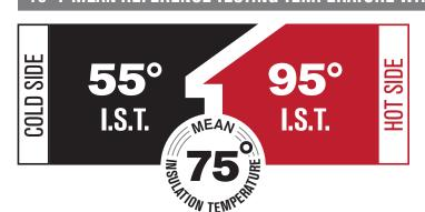
The product standards for most construction insulations require R-value testing at a 75° F mean reference testing temperature with a 40° F temperature differential. The mean reference testing temperature is the mean (average) of the cold side insulation surface temperature (IST) and the hot side insulation surface temperature (IST).
